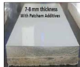
Figure 6: Film appearance of solvent free self leveling epoxy grey high thickness floor coating
