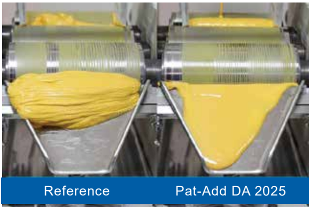
Figure 12. Pat-Add DA 2025 in three-roll mill
